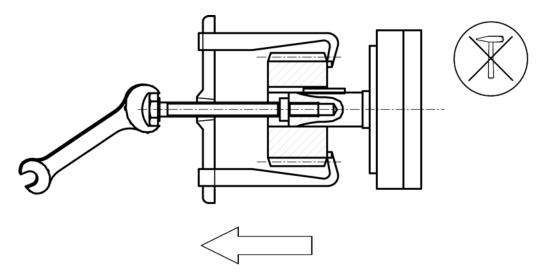
Withdrawing output transmission elements
