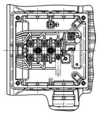
Figure 6-2 Connection to terminal board
