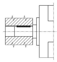
Measures conforming to ISO 10816 must be taken in order to compensate any offset between electrical machines and driven machines.
