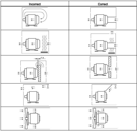
Minimum dimension "x" for the distance between neighboring modules and the air intake of the machine
